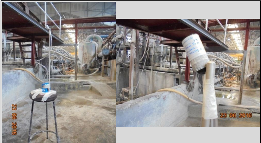
Figure 22: Air sampling of the mixing area – R4
