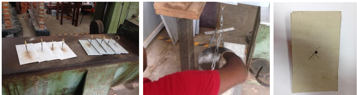
Figure 18: NAIL HEAD PULL THROUGH TEST
