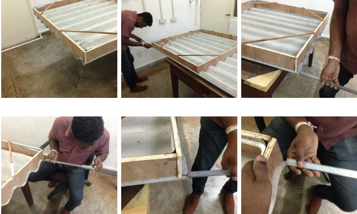
Figure 23: Recording Bending strength of flat sheets
